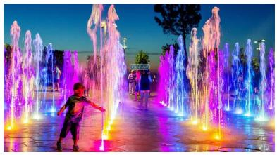
The Smart Dry System is a repeatable, modular and versatile solution that allows to realize dynamic and musical dry fountains of any dimension and of extraordinary water and light effects, since it makes possible to control by DMX protocol each water jet pump and lights individually and independently from the others.
